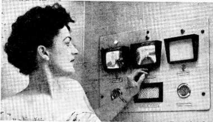
Closed-circuit TV from the front and back doors (with intercom. facilities) and a B.B.C./I.T.A. receiver are incorporated in this bathroom outfit.
